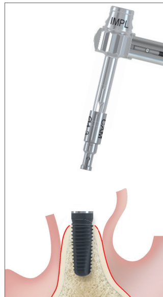
Insertion of the removal adapter to the implant
